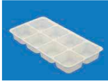
88008 8 Cell Tray O.D.: 6.500 x 3.375 x 0.750 I.D.: 1.375 x 1.375 x 0.750 Mat.: OPS, HIPS
